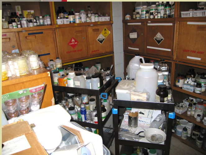
Overcrowded storage closet with carts filled with incompatible chemicals
